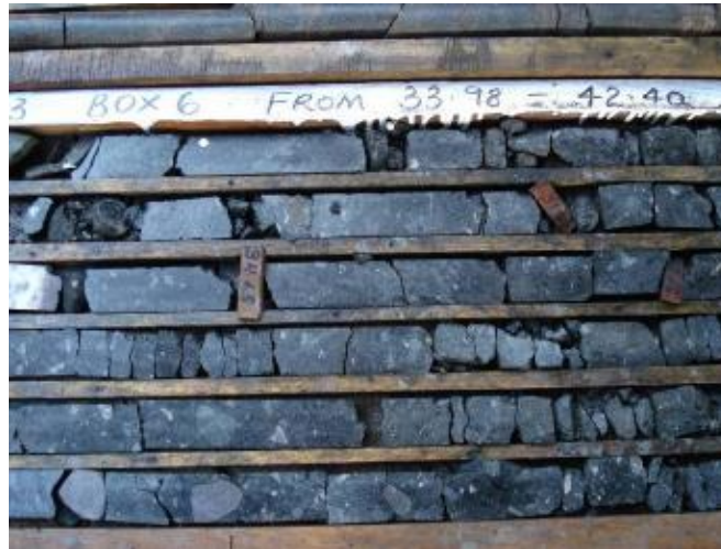
Figure 19: Photo of Drill Core from Borehole PBH 3 at Pandobu Showing Part of Main Kimberlite Intersection with Granite Xenoliths
