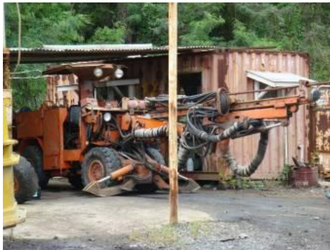
Single Boom Tamrock Drill Rig at Emperor Decline
