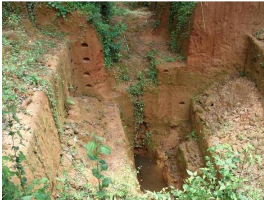
Figure 17: Photo of Mini-Bulk Sample Pit PDS 11 on Kimberlite Dyke at Lalehun
